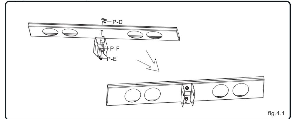
Attach the assembled universal plate to the ceiling mount using the appropriate combination of screws, washers, nut and iron knob. Tighten all screws as shown in fig.4.2.
